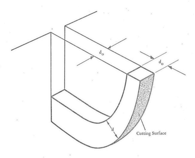
Figure 2. Geometry of the idealized cut.
